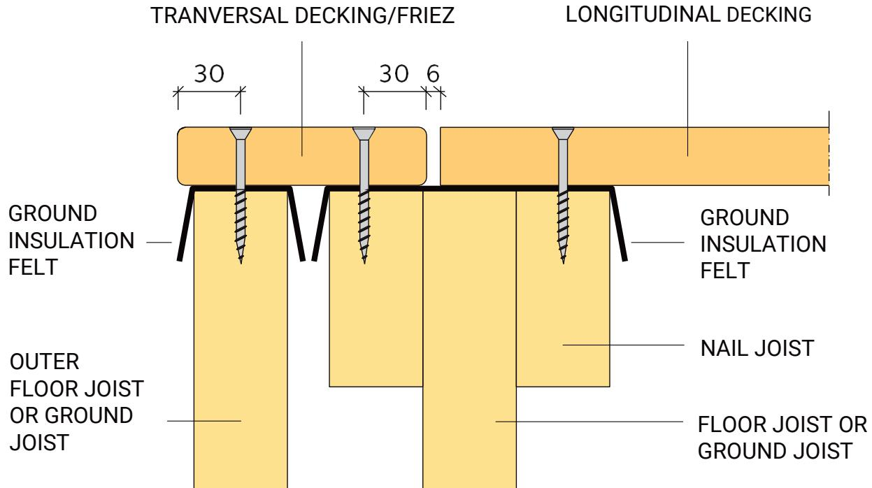
The top of the underlying structure should be protected against moisture by laying longitudinal strips of ground insulation felt, to ensure that the insulation felt runs past the top edges of the floor joists or ground joists by a few centimetres.
