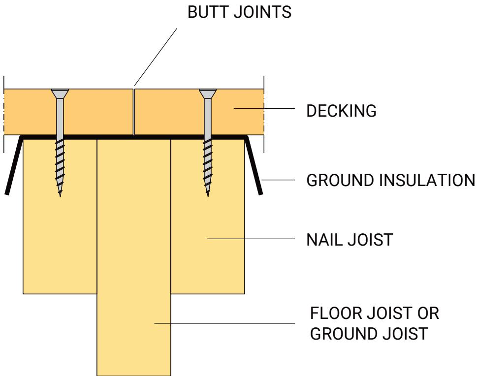
Plan the installation of the decking and select lengths that minimise the number of joints. Joints cannot be avoided across larger areas. Joints must be butted over the supports.
