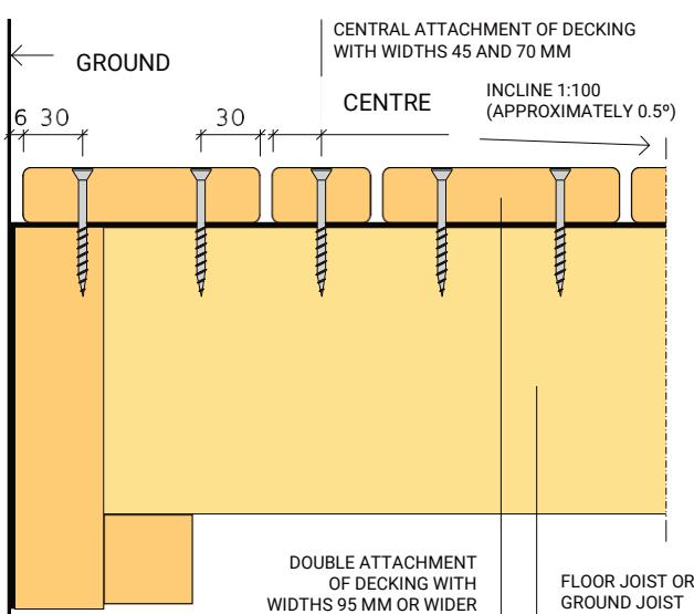
Decking boards with a width of 95 mm or wider must have double attachments and the spacing between the attachment and the edge must be 30 mm. Decking boards with widths of 45 and 70 mm must have centric attachment.
